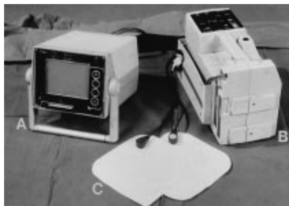
Figure 1 The ECG/impedance cardiogram unit (A) connected to a portable defibrillator (B) and two ECG/defibrillator pads (C).
